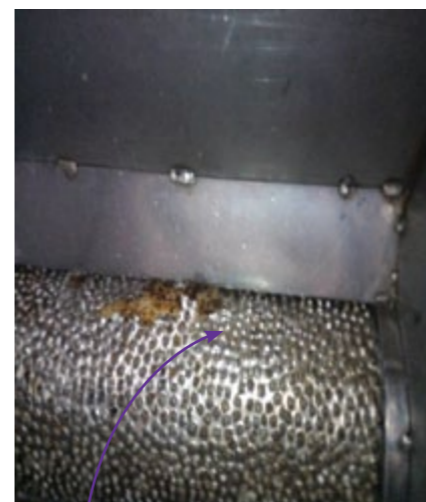
This grater is not in a good condition. Some of the grater brittles have broken off.
